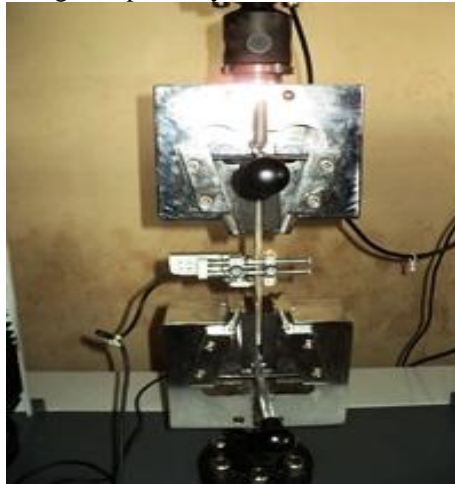
Fig 5: UTM MACHINE (for tensile test)
