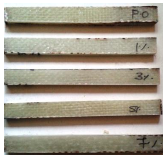
Fig.5: Test Samples of woven fibre with different filler percentage.
