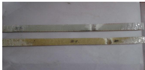
Fig.7: Failure of test specimens under tensile loading (both woven and chopped type with 3% filler)
