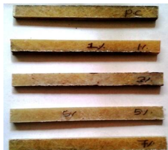
Fig.6: Test Samples of chopped fibre with different filler percentage.
